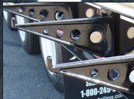
Swing-Out Outriggers with 10" Side Channel
