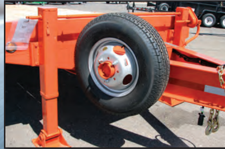
140,000 lb. Twin 2-Speed Jack, Spare Wheel & Tire Mounted
