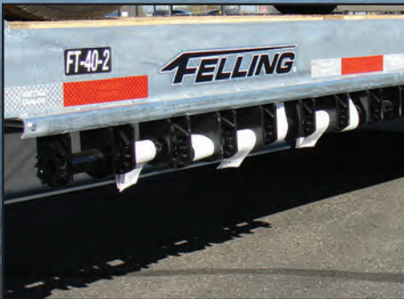
Sliding 4" Belt Winch and Track for Sliding Belt Winch
