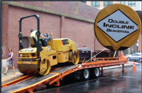
Double Incline Beavertail with Hydraulic Bi-fold Ramps
