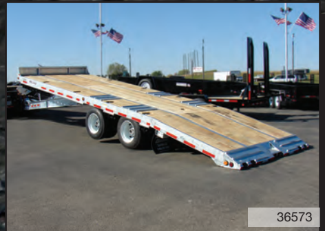
Custom Air Tilt: galvanized, sliding 4" belt winch & track for sliding belt winch, grouser bars over wheels
