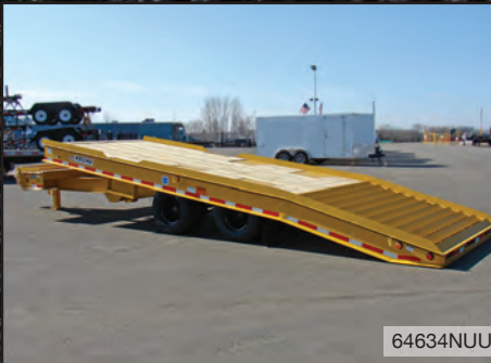
Custom Hyd. Tilt: 2' stationary platform, oak decking w/angle on last 72", custom beavertail, 4" x 3/8" lip up, yellow paint
