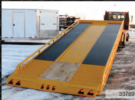
Custom Hyd. Tilt: front 3/4 tread plate, rear 1/2 self-cleaning angle w/oak center, 2" x 2" x 3/16" tube rail along deck, yellow paint
