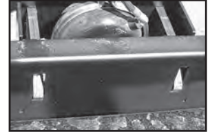
Deck Lock System (only on trailers equipped w/air brakes)
