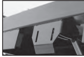
Deck Lock System (only on trailers equipped w/air brakes)
