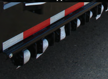
C-Track for Sliding 4" Winch w/ Flat Bar on Opposite Side
