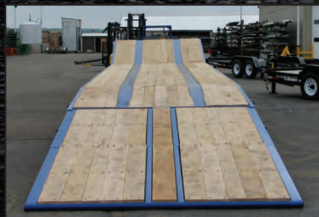
Full Width Wood Inlaid Hydraulic Bi-Fold Ramp
