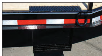
Custom Pullout Side Step with Mesh Traction Aid
