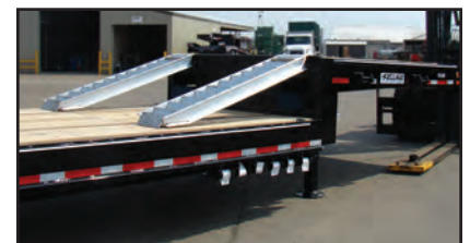
(2) Two Aluminum Ramps with Storage Under Top Deck
