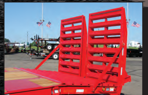
6' x 36" Air Ramp Self Cleaning Angle Upright Ramps
