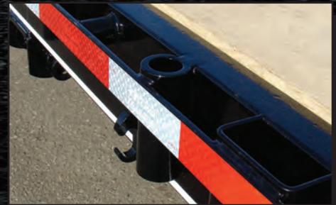
Rub Rail w/Stake Pockets, Pipe Spools, C-Hooks and Pipe Holders
