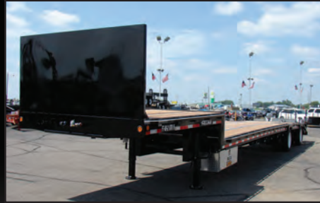
48" Weld-on Solid Bulkhead
