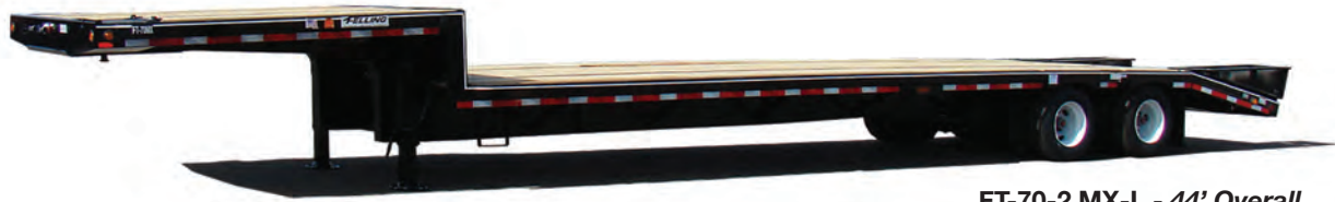
FT-70-2 MX-L - 44' Overall Shown with Std. 90° Neck, 5' Beavertail, 5' Ramps, Optional Stake & Strap with Center Spools
