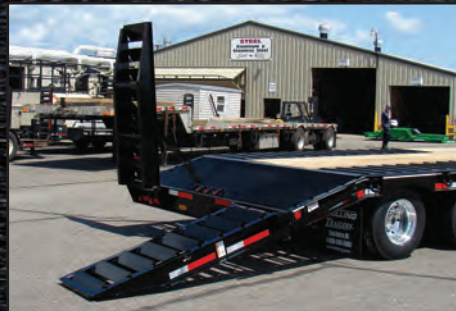
24" x 72" Spring Assist Self Cleaning Stand Up Ramps
