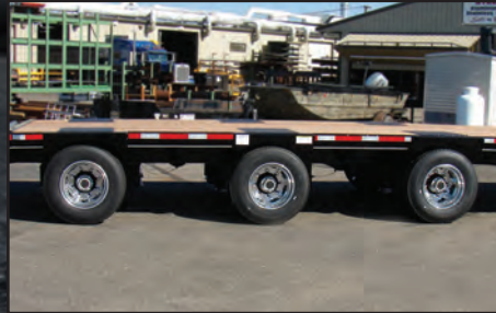
72" Axle Spread with Aluminum Wheels
