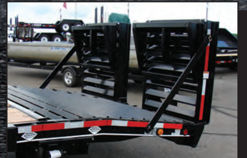
38" x 72" Air Ramp Self Cleaning Upright Ramps with Top Flip-over
