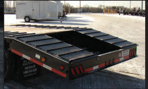
Oil Field Style Beavertail w/ Open Pocket, Steel Covered w/ grouser bars
