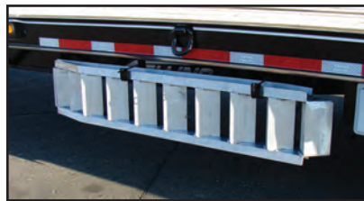
(2) Two Aluminum Ramps with Storage Under Deck
