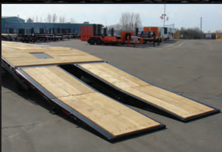
11' Hydraulic Bi-Fold Paver Ramps
