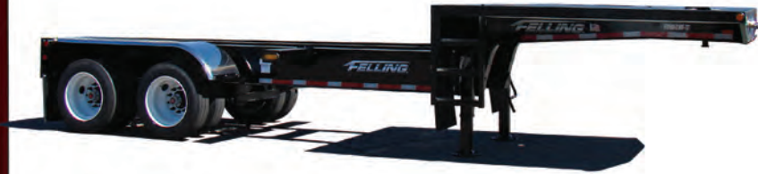
FT-50-2 NN TT - 27' Overall Shown with Optional Tread Plate Top Deck and Aluminum Wheel Fenders
