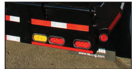
Amber LED Strobe Lights, Switched and Mounted in Tailboard
