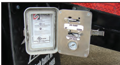
Weather Proof Box for Air Controls and Pressure Gauge
