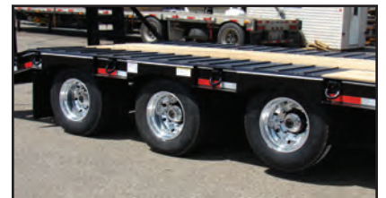
Floor Plate Over Wheels with Traction Bars, Aluminum Wheels and Lift Axle
