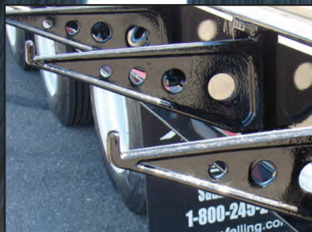
Swing-Out Outriggers with 10" Side Channel
