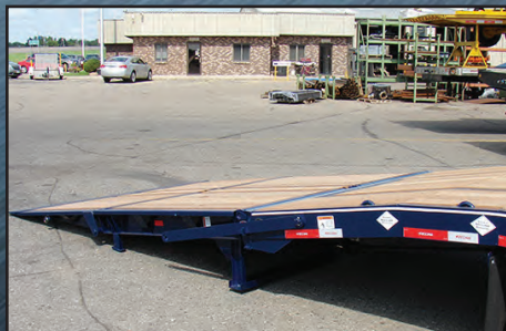
Double Incline Beavertail with Hydraulic Bi-fold Ramps
