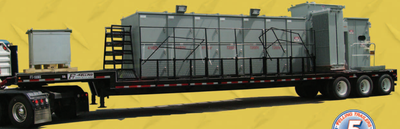
FT-100 MX GEN w/Custom Retractable Catwalk with Handrails & Retractable Stairs
