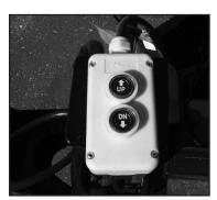
1.) Open the end-gate and secure to trailer prior to raising a loaded body. Ensure that the trailer and tow vehicle are on level ground prior to raising the body. Ensure that ramp tray constraints (if equipped) are secured prior to raising the body. Be careful of any overhead objects prior to raising the body.
