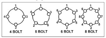
Use a calibrated torque wrench to tighten the fasteners. Verify that wheel studs are free of contaminates such as paint or grease, which may result in inaccurate torque readings. Over-tightening will result in breaking the studs or permanently deforming the mounting stud holes in the wheels, and will void the axle warranty.
