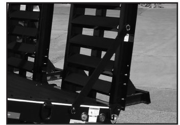
1.) Ramp arm support & cotter key
