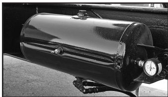
Pressurized Tank on Deck-Over Tilts PSI Pressure Gauge
