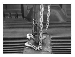
2.) Raise the jack so the gooseneck coupler drops down and attaches to the gooseneck ball.
