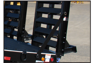
1.) Ramp arm support & cotter key
