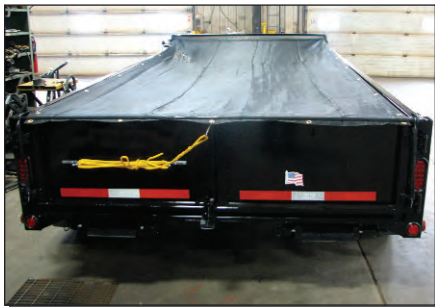
Shown Above: Rear View of Tarp System with tether line securement hooks.
