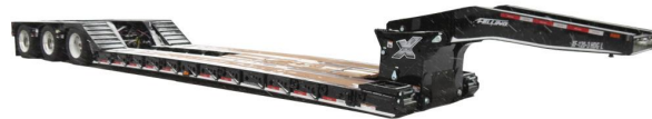
• Shown with optional outrigger boards with hold downs, trunion approach and wheel covers.
